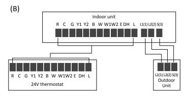
**NOTE:** The wiring method of the thermostat and the internal machine refers to the wiring of the non-communication scheme.
