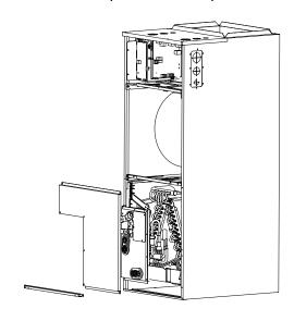
4. Remove T1, T2 temperature sensor plug electronic expansion valve wiring
