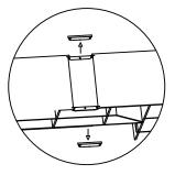
Remove knockouts as shown in the figure.
