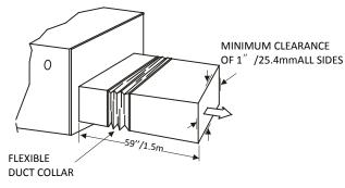
The outlet side pipe length is 59"/1.5m.
