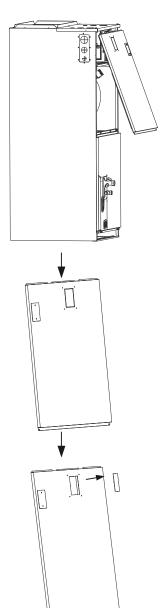
2. Remove the terminal block and power cord, loosen the screws, and remove the electric auxiliary heating cover.
