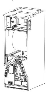
6. Take out the evaporator and drain pan and rotate 180°.
