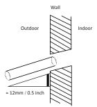
**NOTE:** When drilling the hole, make sure to avoid wires, plumbing, and other sensitive components.
