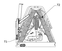
T2: Evaporator central temperature sensor T1: room temperature sensor (some models)
