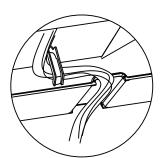
Hook the wire into the buckle and go down from the wire slot.
