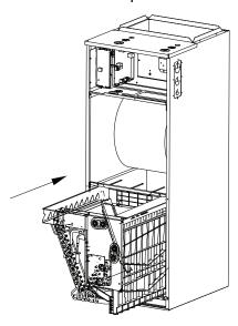
9. Reinstall T1, T2 temperature sensor plug electronic expansion valve and tie up the temperature sensor wires.
