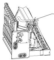
Use cable ties to bind and fix the environmental temperature sensitive bag as shown in the figure.
