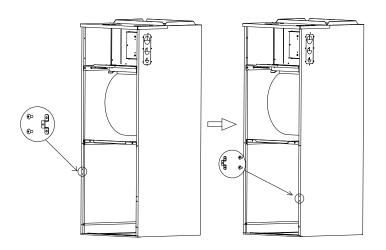
8. Reinstall the evaporator and drain pan.
